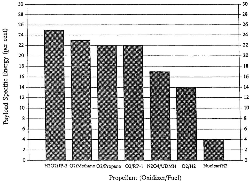
Figure 2: Payload Specific Energy of Candidate Propellants for Single Stage to Orbit
