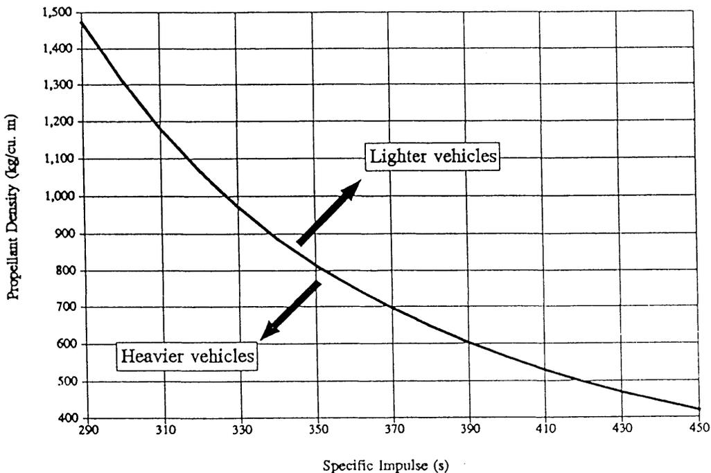
Figure 1: Tradeoffs between density and specific impulse
