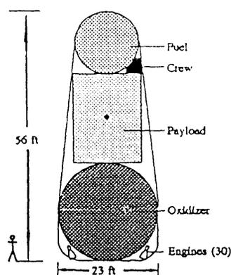
Figure 3: Alternative Single Stage to Orbit Design
